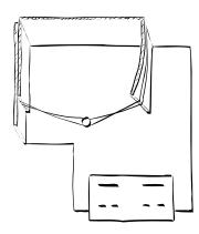
12. Unbend a regular paper clip as illustrated. Put a paper fastener in one switch hole, and secure the paper-clip switch in position with the other paper fastener.
